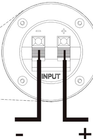
The negative pole, that usually comes with a black wire, has to be hooked into the “-“ connector (left), while the positive pole (usually a red wire) into to the “+“ connector (right). Do not invert the polarities.
